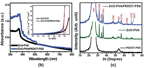
Fig. 2 (a) Energy dispersive X-ray spectrum (EDX) of ZnO nanoparticles embedded in PVA matrix. (b) UV-visible absorption spectra of ZnO-PVA nanocomposite films and ZnO-PVA nanocomposite/PEDOT:PSS heterostructure films.  $(\alpha h v)^2 vs. h v$  plot for ZnO-PVA nanocomposite and ZnO-PVA/PEDOT:PSS heterostructure (inset). (c) X-ray diffraction spectra of PEDOT:PSS, ZnO-PVA nanocomposite and ZnO-PVA nanocomposite/PEDOT:PSS heterostructure grown on PET substrates.
