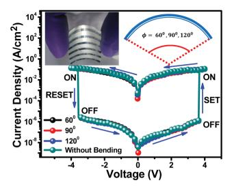
Fig. 6 Current–voltage (I-V) switching characteristic of the S3 memory device. I-V switching characteristic were recorded at  $180^\circ$  (without bending),  $60^\circ$ ,  $90^\circ$  and  $120^\circ$  bending angles of the substrates. Photograph demonstrates the flexibility of a typical S3 memory device (inset).
