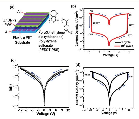
Fig. 3 (a) Schematic diagram of the S3 memory device and molecular structure of PEDOT:PSS films. Current-voltage (I-V) switching characteristics of the (b) S3 memory device, (c) S1 device and (d) S2 device.
