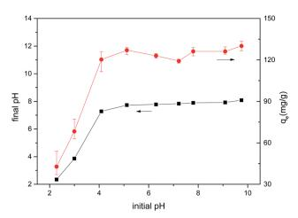
Fig. 6 The effect of initial pH value on the adsorption of MB by CMB (W=0.025 g, T=25 °C, t=80 min, V=20 mL).
