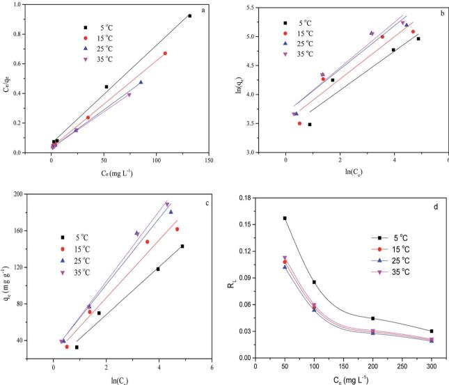
Fig. 8 Linear fits of the adsorption of MB on CMB predicted by various isotherm models. (a) Langmuir; (b) Freundlich; (c) Temkin; (d)  $R_{\rm L}$ .
