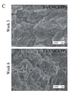
Fig. 3 (A) and (B) DSC and TGA curves of samples. (C) Scanning electron microscopy images of degradation of SA/CMCS and SA/CMCS/PPy hydrogel.
