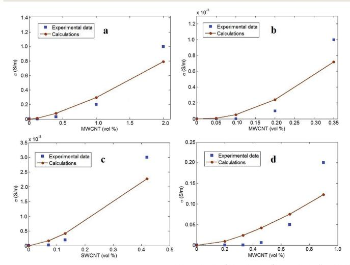
Fig. 2 Experimental results and calculations by the developed model for (a) epoxy/MWCNT, 42 (b) PVC/MWCNT, 43 (c) epoxy/SWCNT 44 and (d) PC/ ABS/MWCNT<sup>45</sup> samples.
