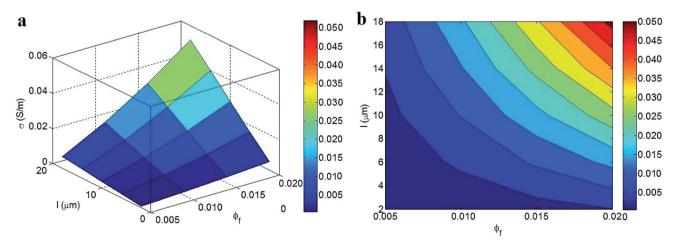
Fig. 3 (a) 3D and (b) contour patterns for the influences of " $\phi_{\rm f}$ " and "l" parameters on the conductivity of nanocomposites at average levels of other variables.
