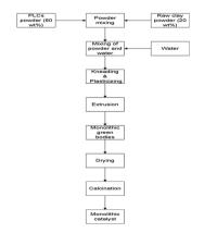
Fig. 2 Schematic representation of extrusion process.
