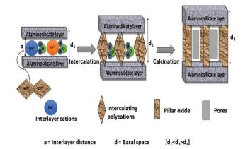
Fig. 1 Schematic representation of clay pillaring process (basal spacing;  $d_1 < d_3 > d_2$ ).
