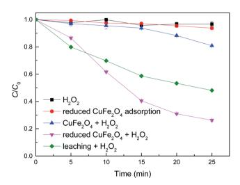
Fig. 4 Comparison of the removal efficiency of MB with different catalytic systems. Conditions:  $[H_2O_2] = 0.5$  mM, catalyst dosage  $0.1 \text{ g L}^{-1}$ , [MB] = 50 mg L<sup>-1</sup>, initial pH =  $3.2 \pm 0.1$ .
