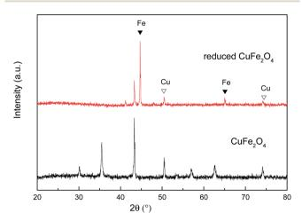
Fig. 2 XRD patterns of CuFe<sub>2</sub>O<sub>4</sub> and reduced CuFe<sub>2</sub>O<sub>4</sub>.
