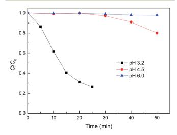
Fig. 5 Effect of initial pH on MB degradation by reduced CuFe<sub>2</sub>O<sub>4</sub>. Conditions:  $[H_2O_2] = 0.5$  mM, [reduced CuFe<sub>2</sub>O<sub>4</sub>] = 0.1 g L<sup>-1</sup>, [MB] =  $50 \text{ mg L}^{-1}$ .
