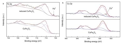
Fig. 3 XPS spectra for Fe 2p (a) and Cu 2p (b) of CuFe<sub>2</sub>O<sub>4</sub> and reduced CuFe<sub>2</sub>O<sub>4</sub>.
