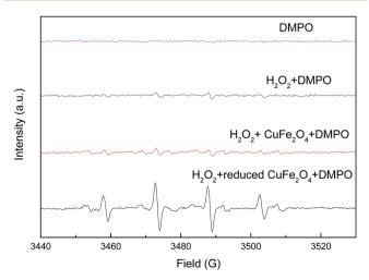
Fig. 11 DMPO spin trapping ESR spectra of 'OH in the systems.
