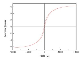
Fig. 9 Magnetization curve of reduced CuFe<sub>2</sub>O<sub>4</sub>.
