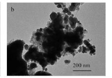
Fig. 1 TEM images of (a) CuFe<sub>2</sub>O<sub>4</sub> and (b) reduced CuFe<sub>2</sub>O<sub>4</sub>.
