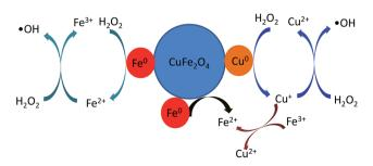
Fig. 12 Schematic diagram of MB degradation mechanism by reduced  ${\rm CuFe_2O_4}.$
