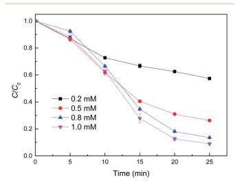
Fig. 7 Effect of  $H_2O_2$  concentration on MB degradation by reduced CuFe<sub>2</sub>O<sub>4</sub>. Conditions: [reduced CuFe<sub>2</sub>O<sub>4</sub>] = 0.1 g L<sup>-1</sup>, [MB] = 50 mg L<sup>-1</sup>, initial pH = 3.2  $\pm$  0.1.
