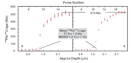
Fig. 6 Consecutive laser pulse analyses of two zoned zircon grains are shown in (a) and (b), indicating that LA-MC-ICP-MS with a MIC system can be applied to isotopic depth profile analysis with a high depth resolution of  $\sim 0.1 \,\mu m$  per pulse (modified from ref. 73).
