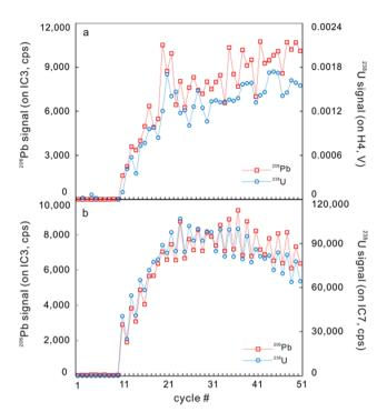
Fig. 5 A typical time-resolved profile on GJ-1 zircon for continuous laser ablation analysis measured on a Neptune Plus. (a) Signals of <sup>206</sup>Pb (red) and <sup>238</sup>U (blue) were counted on IC3 and Faraday cup H4, respectively. (b) Signals of <sup>206</sup>Pb (red) and <sup>238</sup>U (blue) were counted on IC3 and IC7, respectively (from ref. 5).
