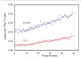
Fig. 2 The measured  $^{206}\text{Pb}/^{238}\text{U}$  ratios of zircon reference materials 91500 (in blue) and GJ-1 (in red) by LA-MIC-ICP-MS show that the ratio is stable to a depth of about 1.3  $\mu$ m (approx. 10 pulses and 130 nm per pulse) and then increases as the ablation continues (G2 laser ablation system at a laser fluence of 4 J cm<sup>-1</sup>, repetition rate of 4 Hz and beam size of 5  $\mu$ m).
