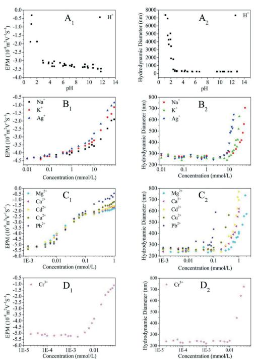
Fig. 7 Electrophoretic mobility (EPM) and hydrodynamic diameter of GO as a function of the cation concentration of  $H^+$  ( $A_1$  and  $A_2$ ), monovalent metal cations ( $B_1$  and  $B_2$ ), divalent metal cations ( $C_1$  and  $C_2$ ), and trivalent metal cations ( $D_1$  and  $D_2$ ). Reprinted with permission from ref. 71. Copyright 2016, American Chemical Society.
