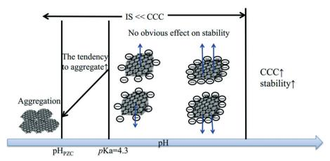
Fig. 6 Diagrams of the impact of pH on GO stability.
