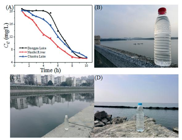
Fig. 20 (A) Sedimentation kinetics of GO sheets in the three natural surface waters collected from Dongpu Lake (B), Nanfei River (C), and Chaohu Lake (D).<sup>67</sup> Reprinted with permission from ref. 67. Copyright 2017, Elsevier.
