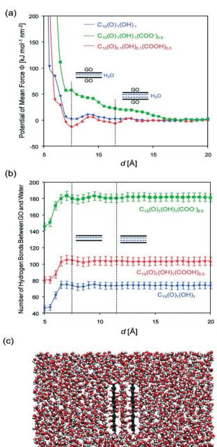
Fig. 5 Simulated (a) potential of the mean force between two parallel, fixed GO sheets, and (b) the number of H-bonds formed between the two sheets and the surrounding water molecules as a function of the intersheet separation, d. Three forms of GO  $[C_{10}(O)_1(OH)_1, C_{10}(O)_1(OH)_1, C_{10}(O)_1(OH)_1, C_{10}(O)_1, C_{10}$
