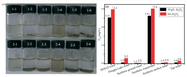
Fig. 21 (A) Visual images of GO in the absence and presence of  $Al_2O_3$  in different waters. (B) Concentrations of the residual GO sheets in the supernatant as a function of cation types and concentrations in the absence and presence of  $Al_2O_3$  in natural and synthetic waters.  $C_{(GO)initial} = 6$  mg L<sup>-1</sup>, m/V = 10 g L<sup>-1</sup> (i.e.,  $Al_2O_3$  concentration). Reprinted with permission from ref. 84. Copyright 2014, American Chemical Society.
