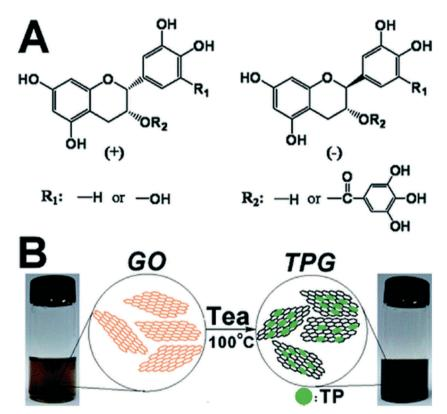
Fig. 26 (A) Chemical structure of tea polyphenols (TPs). (B) Schematic illustration of the preparation of TP reduced graphene. 185 Reprinted with permission from ref. 185. Copyright 2011, American Chemical Society.
