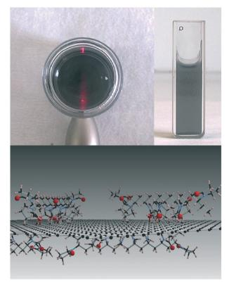
Fig. 17 Top: The Tyndall scattering effect is seen in the left image for the aqueous colloidal dispersion of graphite after settling and centrifugation (0.1 mg ml<sup>-1</sup>). The cuvette on the right shows the optical transparency of the same dispersion. Bottom: Schematic model of polyvinylpyrrolidone-coated graphene. 127 Reprinted with permission from ref. 127. Copyright 2009, Elsevier.
