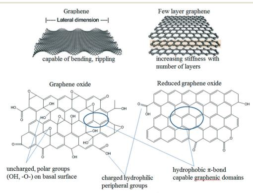
Fig. 2 Examples of GAs and selected properties relevant to their colloidal behavior. 12,14 Reprinted with permission from ref. 12. Copyright 2014, American Chemical Society. Reprinted with permission from ref. 14. Copyright 2012, American Chemical Society.
