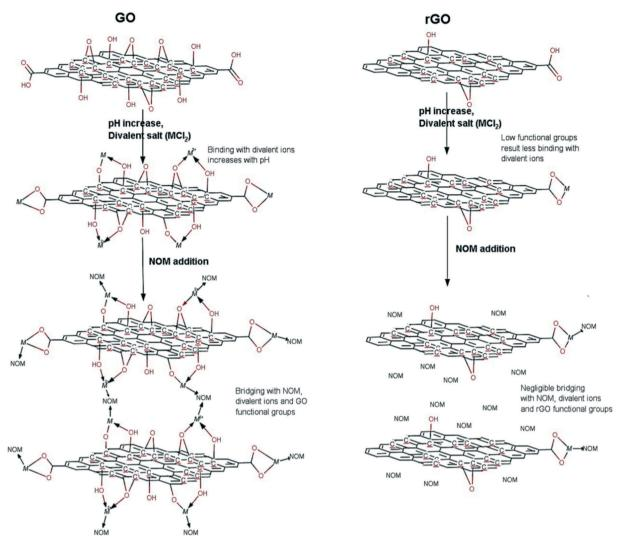
Fig. 3 Interaction mechanisms of pH, divalent cations (M: Ca<sup>2+</sup>, Mg<sup>2+</sup>) and natural organic matter (NOM) with GO and rGO.<sup>55</sup> Reprinted with permission from ref. 55. Copyright 2015, American Chemical Society.
