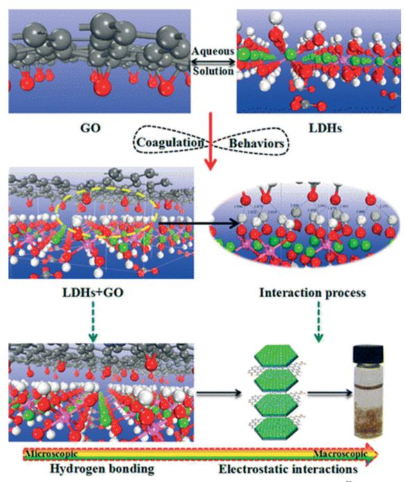
Fig. 14 Optimized geometrical structures and coagulation processes of GO on layered double hydroxides (LDHs). Permission from ref. 99. Copyright 2016, American Chemical Society.
