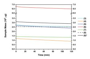
Fig. 6 Mass loss (mg) for complexes 3–8 over 120 min at 120 °C and 160 °C\*.
