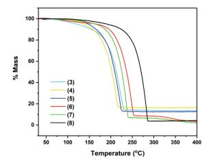
Fig. 5 Thermogravimetric analysis data for complexes 3-8.
