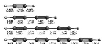
**Fig. 1** AE-CCSD(T)/cc-pCVQZ equilibrium geometries (Å) for  $HC_{2n}H$ . Experimentally determined equilibrium bond lengths for acetylene,  $^{87}$  diacetylene,  $^{53}$  and triacetylene  $^{88}$  are given in italics below.
