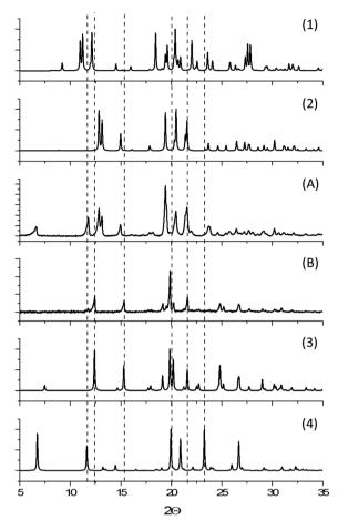
Fig. 6 (A) XRPD pattern of ε-CPA after impact treatment with heptane, (B) XRPD pattern of  $\beta$ -CPA converted into  $\gamma$ -form after shear treatment with heptane, and simulated XRPD patterns for (1)  $\beta$ -CPA, (2)  $\epsilon$ -CPA, (3)  $\gamma$ -CPA and (4)  $\delta$ -CPA
