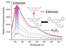
Fig. 6 Fluorescence spectra of **Pinkment-OAc** (0.5 μM) following incubation (15 min) with PLE (0.1–0.6 U) and subsequent addition of H<sub>2</sub>O<sub>2</sub> (1 mM). The data was collected in PBS buffer (100% w/w H<sub>2</sub>O) at pH = 7.4, 25 °C.  $\lambda_{\rm ex}$  = 545–20 nm. Dashed line represents H<sub>2</sub>O<sub>2</sub> (1 mM) addition only.
