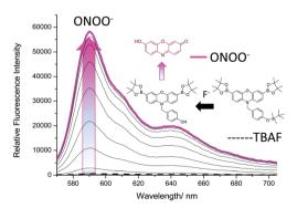
Fig. 3 Fluorescence spectra of Pinkment-OTBS (0.5  $\mu\text{M})$  with addition of TBAF (10 mM) and incubated for 1 h and then measured. Followed by incremental additions of ONOO $^-$  (0–20  $\mu$ M) The data was obtained in PBS (52% w/w MeOH:  $H_2O$ ), pH = 8.2 at 25 °C.  $\lambda_{ex}$  = 545–20 nm. Dashed line represents TBAF (10 mM) addition only.
