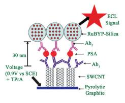
Fig. 11 Scheme of representation of ECL-based SWCNT immunosensors after addition of PSA and  $[Ru-(bpy)_3]^{2^+}$ -silica-Ab<sub>2</sub> nanoparticles. (Reprinted with permission from ref. 63. Copyright 2009 Royal Chemical Society.)
