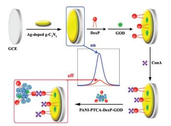
Fig. 20 The illustration of the synthetic process of (A)  $Ag-g-C_3N_4$  and (B) PANI-PTCA-DexP-GOD, and (C) the preparation of the ECL biosensor. (Reprinted with permission from ref. 89. Copyright 2016, Elsevier.)
