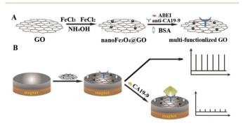
Fig. 5 Schematic diagram for (A) the preparation of multi-functionalized graphene oxide, and (B) the fabrication and application protocol of the ECL immunosensor using multi-functionalized graphene oxide. (Reprinted with permission from ref. 47. Copyright 2015 Elsevier.)
