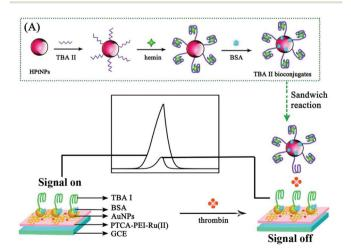
Fig. 2 Schematic illustration of the possible luminescence mechanism of the "on-off" ECL aptasensor. (Reprinted with permission from ref. 9. Copyright 2015 American Chemical Society.)
