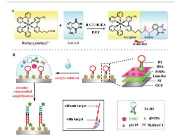
Fig. 4 Representations of (A) the synthesis of the Lum-Ru compounds and (B) fabrication of the aptasensor and the reaction mechanism. (Reprinted with permission from ref. 18. Copyright 2017 Wiley.)
