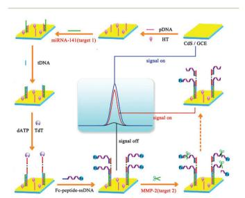
Fig. 33 Fabrication of an ECL biosensing platform for the detection of multiple types of biomarkers on a single interface. (Reprinted with permission from ref. 157. Copyright 2017 American Chemical Society.)
