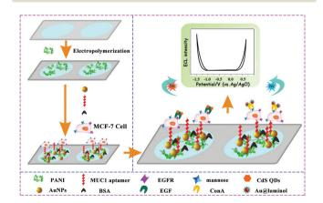
Schematic Fig. 31 Preparation and Illustration of Electrochemiluminescence Signal System. (Reprinted with permission from ref. 154. Copyright 2017 American Chemical Society.)
