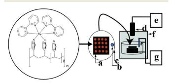
Fig. 30 Conceptual diagram of the ECL array instrumentation. RuPVP polymer, DNA, and enzymes are located at each spot on a (a) pyrolytic graphite block; with (b) Ag/AgCl reference electrode, (c) Pt wire counter electrode, (d) CCD camera, (e) computer, (f) gel-doc dark room, and (g) potentiostat for applied voltage control. (Reprinted with permission from ref. 147. Copyright 2007, American Chemical Society.)
