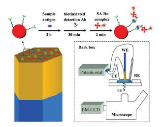
Fig. 29 (Top) A sandwich immunoassay is performed by exposing antibody-functionalized microbeads to three solutions. The beads are housed in microwells created from an etched gold-coated fiber-optic bundle. The gold coated fiber bundle acts as the working electrode (WE) for ECL. CE and RE refer to counter electrode and reference electrode. (Reprinted with permission from ref. 144. Copyright 2009, American Chemical Society.)
