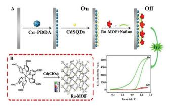
**Fig. 6** (A) Schematic illustration of the ECL sensor. (B) Preparation of the Ru-MOF. (Reprinted with permission from ref. 48. Copyright 2017 Elsevier.)
