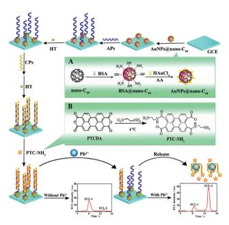
Fig. 22 Schematic illustration of the preparation process of the ratiometric aptasensor: inset of (A) and (B) display the preparation procedure of AuNPs@nano-C60 and PTC-NH2. (Reprinted with permission from ref. 14. Copyright 2015, American Chemical Society.)
