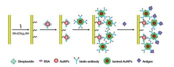
Fig. 13 Schematic illustration of the fabrication processes of the labelfree ECL immunosensor using luminol-AuNPs as antibody carriers and sensing platform. (Reprinted with permission from ref. 67. Copyright 2013 Royal Chemical Society.)
