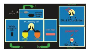
**Fig. 36** Schematic diagram of the working principle of a m-s-OECLD. f: Front sheet; b1: the sheet folded to the back first; b2: the back sheet. (Reprinted with permission from ref. 165. Copyright 2013 The Royal Society of Chemistry.)
