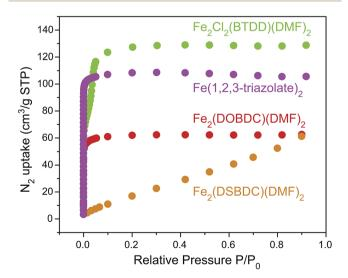
Fig. 6  $N_2$  adsorption isotherms (77 K) of Fe<sub>2</sub>(DOBDC)(DMF)<sub>2</sub>, Fe<sub>2</sub>(DSBDC)(DMF)<sub>2</sub>, Fe<sub>2</sub>Cl<sub>2</sub>(BTDD)(DMF)<sub>2</sub>, and Fe(1,2,3-triazolate)<sub>2</sub>.
