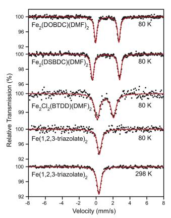
Fig. 4  $^{57}$ Fe Mössbauer spectra of Fe<sub>2</sub>(DOBDC)(DMF)<sub>2</sub>, Fe<sub>2</sub>-(DSBDC)(DMF)<sub>2</sub>, and Fe<sub>2</sub>Cl<sub>2</sub>(BTDD)(DMF)<sub>2</sub> at 80 K as well as Fe(1,2,3-triazolate)<sub>2</sub> at 80 and 298 K. All samples were kept in N<sub>2</sub> atmosphere. Black dots represent experimental data, and red curves represent Lorentzian fitting curves.
