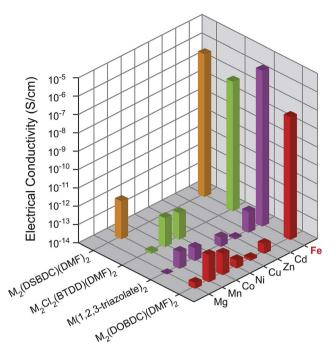
Fig. 2 Electrical conductivity in  $M_2(DOBDC)(DMF)_2$ ,  $M_2-(DSBDC)(DMF)_2$ ,  $M_2Cl_2(BTDD)(DMF)_2$ , and  $M(1,2,3-triazolate)_2$  measured at 300 K, in  $N_2$  atmosphere, and in the dark.
