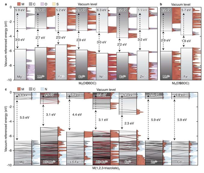
Fig. 7 Calculated energy bands and projected density of states (PDOS) of (a) M<sub>2</sub>(DOBDC), (b) M<sub>2</sub>(DSBDC), and (c) M(1,2,3-triazolate)<sub>2</sub>. The electron energies are referenced to the vacuum level using the method presented in ref. 33. E<sub>VBM</sub> are shown on the top and band gaps are shown in the middle of each sub-figure.
