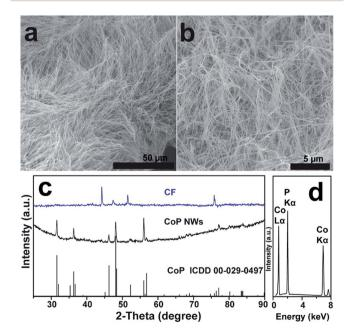
Fig. 1 (a and b) SEM images of CoP NWs. (c) XRD patterns of the CoP NW electrode and bare Co foam (CF). The standard ICDD powder diffraction pattern of CoP (No. 00-029-0497) is also given for reference. (d) EDX spectrum of CoP NWs. The CoP NW electrode was obtained upon thermal phosphorization at 600 °C.
