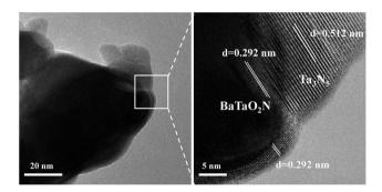
Fig. 3 Representative TEM (left) and locally enlarged HRTEM (right) images of the chosen Ba(0.3)-Ta<sub>3</sub>N<sub>5</sub> sample.
