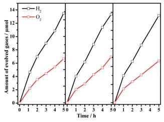
Fig. 5 Multiple cycles of Z-scheme overall water splitting with 0.5 wt% Pt/Ba(0.3)– $Ta_3N_5$  and 0.45 wt% PtO<sub>x</sub>/WO<sub>3</sub> as H<sub>2</sub>-evolving and O<sub>2</sub>-evolving photocatalysts, respectively. Reaction conditions: 50 mg of Pt/Ba(0.3)– $Ta_3N_5$  and 50 mg of PtO<sub>x</sub>/WO<sub>3</sub>; 100 mL of Nal aqueous solution (1.0 mM); 300 W xenon lamp ( $\lambda$  > 420 nm), top-irradiation.
