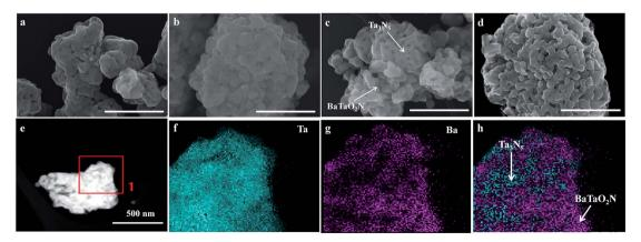
Fig. 2 FESEM images of typical samples: (a)  $Ta_3N_5$ , (b)  $BaTaO_2N$ , (c) a mixture of  $Ta_3N_5$  and  $BaTaO_2N$ , and (d)  $Ba(0.3) - Ta_3N_5$  (the scale bar is 500 feets). nm). Elemental mappings of Ba(0.3) –  $Ta_3N_5$ : (e) TEM image, (f) Ta element, (g) Ba element, and (h) simulated dispersion of  $Ta_3N_5$  and  $Ta_3N_5$  and
