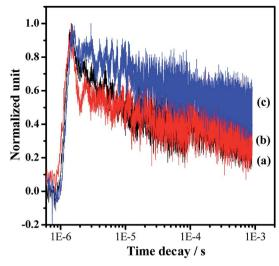
Fig. 6 Normalized transient absorption profiles of the representative samples in a vacuum: (a) Pt/Ta $_3$ N $_5$ , (b) Pt/BaTaO $_2$ N and (c) Pt/Ba(0.3)— Ta $_3$ N $_5$ . The pulse laser at 355 nm was used to excite the samples for the IR tests. The cocatalyst of Pt with a loading amount of 0.5 wt% was deposited by impregnation and a subsequent H $_2$  reduction method.
