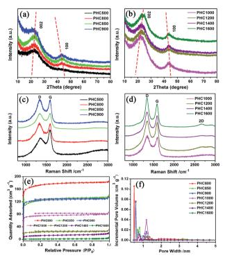
Fig. 2 Structure of PHC carbonized at different temperature. (a, b) XRD patterns; (c, d) Raman spectra; (e) N<sub>2</sub> adsorption-desorption isotherms; (f) pore size distribution calculated by the BJH method
