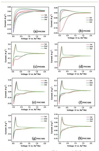
Fig. 4 (a-h) Cyclic voltammetry (CV) curves of PHC electrodes carbonized at different temperature.
