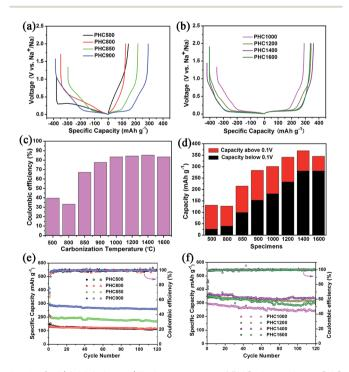
Fig. 5 (a, b) Initial charge/discharge curves of PHC electrodes at 0.1C (30 mA  $\rm g^{-1}$ ); (c) initial coulombic efficiency of PHC electrodes; (d) specific capacity from plateau and slope contributions of PHC electrodes; (e, f) cycling performance at 0.1C at room temperature.
