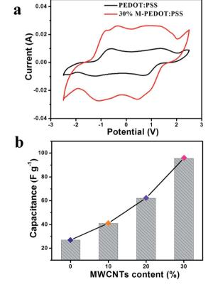
Fig. 4 (a) Cyclic voltammetry (CV) curves for the PEDOT:PSS and 30% M-PEDOT:PSS electrode based actuators at  $100 \text{ mV s}^{-1}$  sweep rate. (b) The calculated capacitances for actuators.
