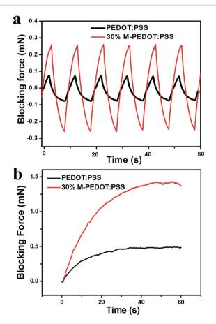
Fig. 7 Blocking force of PEDOT:PSS and 30% M-PEDOT:PSS electrode based actuators (a) under 2.5 V at 0.1 Hz. (b) under 2.5 V DC
