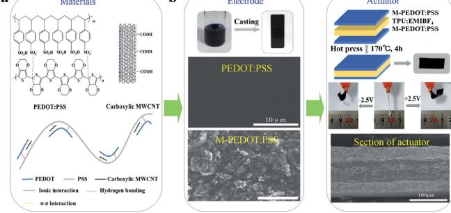
Fig. 1 Schematic illustration of actuator based on M-PEDOT:PSS electrode and fabricated by hot press
