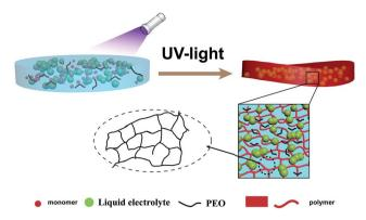
**Scheme 1** The preparation process and the illustration of the GPE membrane.
