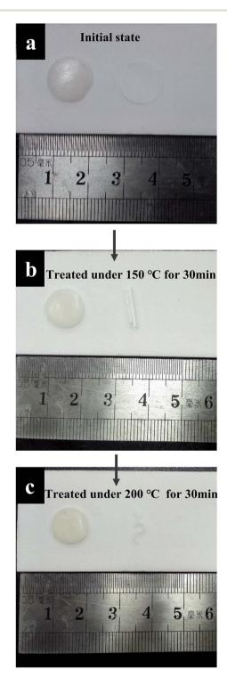
Fig. 2 Photo image of GPE and commercial separator (a) initial state, (b) heat treatment at 150  $^{\circ}$ C for 30 min and (c) further heat treatment at 200 °C for 30 min.
