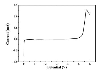
Fig. 5 Linear sweep voltammogram of the gel polymer electrolyte at 0.5 mV s $^{-1}$ .
