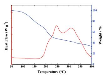
Fig. 4 Thermogravimetric analysis and Differential Scanning Calorimetry (DSC) curves of the gel polymer electrolyte.
