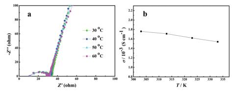
(a) EIS plots of SS/GPE/SS at different temperatures and (b) ionic conductivity of the GPE at different temperatures
