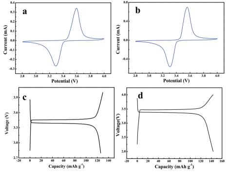
Fig. 9 (a) CV curve of LiFePO<sub>4</sub> testing with GPE. (b) CV curve of LiFePO<sub>4</sub> cathode with liquid electrolyte. (c) Charge–discharge curves of LiFePO<sub>4</sub> testing with GPE at 80 mA  $g^{-1}$ . (d) Charge–discharge curves of LiFePO<sub>4</sub> testing with liquid electrolyte at 80 mA  $g^{-1}$ .
