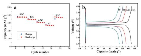
Fig. 11 (a) Charge-discharge curves of Li/GPE/LiFePO<sub>4</sub> at varying currents from 16 mA q<sup>-1</sup> (0.1C) to 160 mA q<sup>-1</sup> (1C). (b) Discharge capacities of Li/SPE/AQ at different currents.
