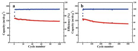
Fig. 10 Cycling performance of LiFePO<sub>4</sub>/GPE/Li battery testing at current density of (a) 0.5C, (b) 0.2C.
