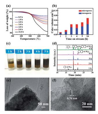
Fig. 4 (a) Time-dependent TGA analysis of the spent Zn/ZSM-12 catalyst used in the MTA reaction. (b) Pore volume of ZSM-12 after different reaction times. (c) Photographs of the spent catalysts after being dissolved in 15% HF and extracted by CH2Cl2. (d) GC-MS chromatograms of the organic species in the spent catalysts extracted by CH<sub>2</sub>Cl<sub>2</sub>. (e) and (f) TEM images of the remaining carbon structure after using 15% HF solution to dissolve the spent Zn/ZSM-12 catalyst.
