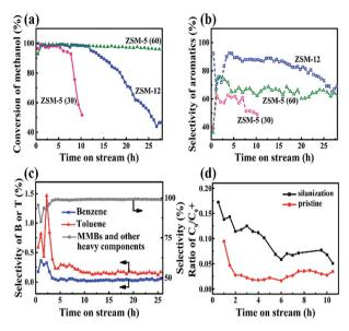
Fig. 3 (a) Time-dependent methanol conversions of Zn/ZSM-12, Zn/ ZSM-5 (30) and Zn/ZSM-5 (60). (b) Selectivity of aromatics for Zn/ZSM-12, Zn/ZSM-5 (30) and Zn/ZSM-5 (60). (c) Selectivity of B, T and MMBs (and other heavy components) in aromatics using Zn/ZSM-12. (d) Ratio of  $C_9/C_9^+$  with the catalyst, with or without silanization at different reaction times.
