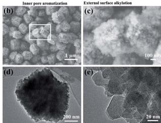
Fig. 1 (a) Proposed technical route for the preparation of multimethylbenzenes from methanol using a nano ZSM-12 zeolite-based catalyst. (b) SEM image of H-ZSM-12. (c) High-resolution SEM image of H-ZSM-12. (d) TEM image of H-ZSM-12. (e) High-resolution TEM image of H-ZSM-12.
