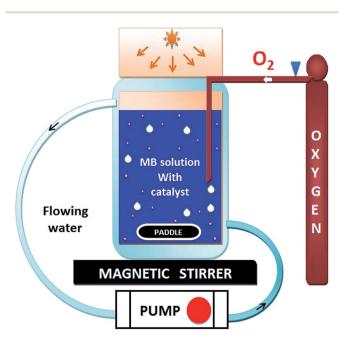
Fig. 1 Schematic representation of the used photocatalytic reactor setup
