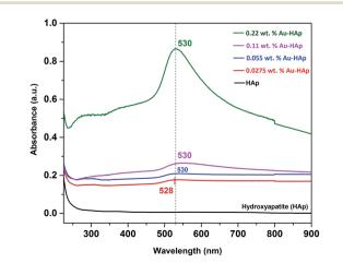
Fig. 3 UV-Vis DRS spectra of HAp nanoparticles loaded with Au in different weight percentages.
