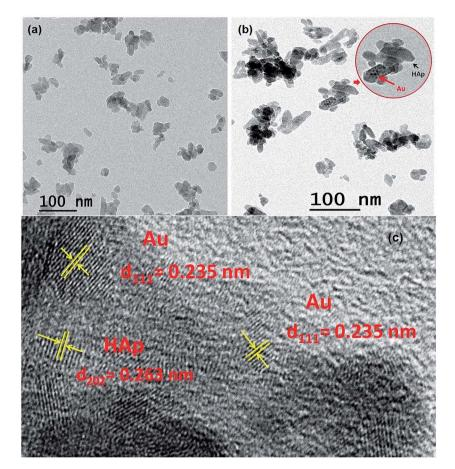
Fig. 6 Typical (a) TEM image of HAp, (b) 0.055 wt% Au-HAp, and (c) HRTEM image of 0.055 wt% Au-HAp samples. Formation of Au nano-particles of 2 to 6 nm sizes at the surface and inter-particle spaces of the nanocomposite is clear from the HRTEM image.
