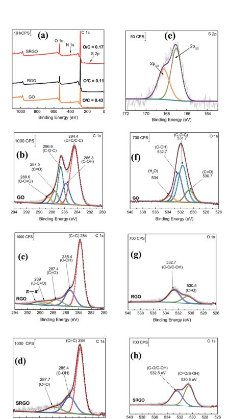
Fig. 7 (a) XPS survey spectra of graphene oxide (GO), reduced graphene oxide (RGO) and sulfophenyl-modified RGO (SRGO); XPS C 1s spectra of (b) GO, (c) RGO and (d) SRGO, (e) S 2p core level spectrum of SRGO and XPS O 1s spectra of (f) GO, (g) RGO and (h) SRGO.
