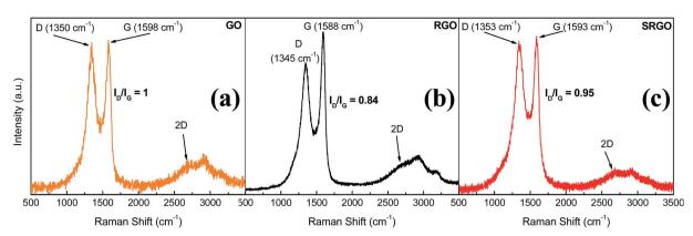
Fig. 6 Raman spectra of GO, RGO and SRGO recorded using 532 nm laser excitation.
