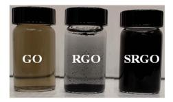
Fig. 1 Optical images of GO, RGO and SRGO dispersed in water at the concentration of 0.5 mg  $\,\mathrm{mL}^{-1}$ .
