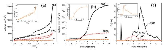
Fig. 4 (a)  $N_2$  adsorption isotherms of graphene oxide, reduced graphene oxide before (RGO) and after reaction with *in situ*-generated 4-sulfophenyl diazonium cations (SRGO), (b) cumulated surface area vs. pore width of GO, RGO and SRGO, (c) pore size distribution of GO, RGO and SRGO. The insets present the data for GO at a more sensitive scale.
