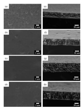
Fig. 4 Top view (a–d) and cross-section (e–h) SEM images of the PI membrane (a and e) and GO/PI MMMs with 0.5 wt% (b and f); 1 wt% (c and q), 2 wt% (d and h) GO loading.
