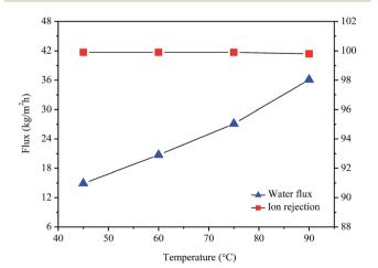
Fig. 6 Water flux and ion rejection of the GO/PI MMMs with 1 wt% GO loading as a function of the operation temperature for desalination of 3.5 wt% seawater by pervaporation.
