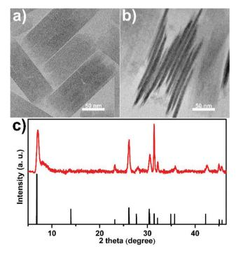
Fig. 1 (a, b) TEM images and (c) XRD pattern of the as-synthesized CeO (CH<sub>3</sub>COO) ML nanoplates, the reference pattern in (c) is produced from ref. 41 and 52.
