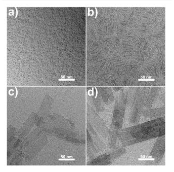
Fig. 2 TEM images of products obtained at (a) 1 min, (b) 3 min, (c) 5 min and (d) 10 min after injection during the synthesis of CeO (CH<sub>3</sub>COO) ML nanoplates.
