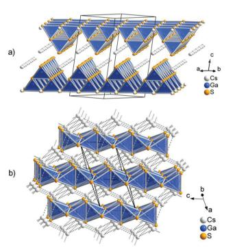
Fig. 1 (a) Anionic layers in  $CsGaS_2-mC64$ . (b) Crystal structure of  $CsGaS_2-mC16$ , showing the arrangement of the anionic chains in the diamond-like topological arrangement of the  $Cs^+$  cations (dashed lines).
