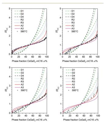
**Fig. 6** Plot of  $\alpha$  against  $t/t_{0.5}$  for all measured temperatures (transparent dots) used for the determination of the crystallisation mechanism (lines) according to literature.16
