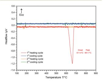
Fig. 2 Differential thermal analysis (DTA) of CsGaS<sub>2</sub>-mC64 (the baseline was manually subtracted). Two heating- and cooling cycles (heating-/ cooling rate 10 °C min<sup>-1</sup>) reveal an irreversible phase-transition.
