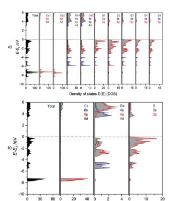
Fig. 10 Calculated total (TDOS) and partial density of states (PDOS) for (a) CsGaS<sub>2</sub>-mC64 and (b) CsGaS<sub>2</sub>-mC16.
