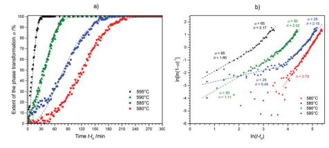
Fig. 5 (a) Progression of the phase fraction of  $CsGaS_2-mC16$  during the isothermal measurements (dashed lines indicate a fit based on the Avrami equation using the determined kinetic parameters n and K). (b) Sharp–Hancock plots for the different experiments (dashed lines indicate a linear fit for the determination of n and K).
