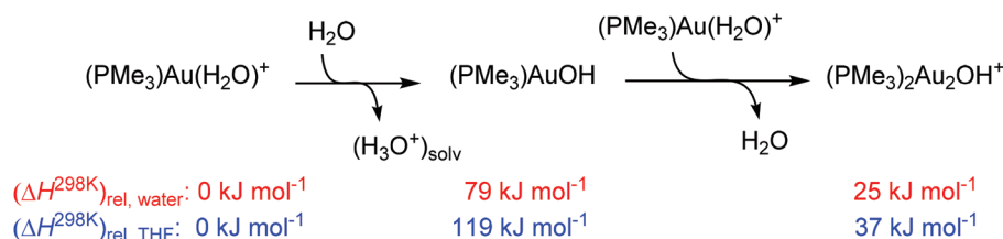
Scheme 2 Reaction of [(PMe 3 )Au(H 2 O)] + with water.
