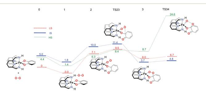
Fig. 4 Calculated reaction profile for the first part of the catechol dioxygenation mechanism, starting from the  $[Fe(LN_4H_2)(Cat)]^+$  complex 0. Electronic energies (kcal mol<sup>-1</sup>), obtained using the S12g/TZ2P level of theory, are given relative to reactants.
