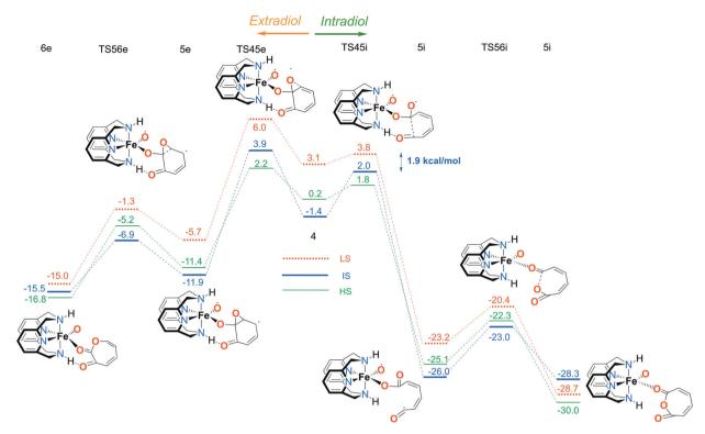
Fig. 5 Calculated reaction profile for the second part of the catalytic mechanism with the LN<sub>4</sub>H<sub>2</sub> ligand, branching to the extradiol (left) and intradiol (right) pathways. Electronic energies (kcal mol<sup>-1</sup>), obtained using the S12g/TZ2P level of theory, are given relative to reactants.
