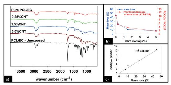
Fig. 5 (a) ATR-FTIR analysis of the nanocomposites shows a reduction in intensity of the ester peak (1720 cm<sup>-1</sup>) following 125 days irradiation. (b) Following 125 days of exposure, the final mass loss and fractional decrease of ester band area show a similar dependence on CNT loading. (c) Mass loss increases linearly with the fractional decrease in ester band area.
