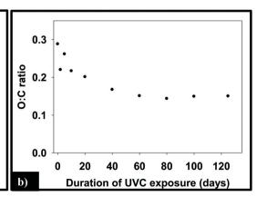
Fig. 4 Transformations in (a) the C(1s) region and (b) O:C ratio of the 1.5% CNT composites as a function of UVC irradiation. The largest changes are seen to occur during the by first 20–40 days with little change in either the C(1s) region or the O:C ratio thereafter.
