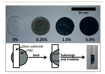
Fig. 1 (Top) Polymer nanocomposites (PNC) prepared by solution blending with a poly- $\epsilon$ -caprolactone (PCL) polymer matrix and 0–5% (by weight) SWCNT nanoparticle filler. (Bottom) Samples are bound to a glass slide using Teflon tape, submerged in water, and irradiated in a quartz test tube.
