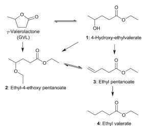
Fig. 27 Reaction pathways of GVL conversion in ethanol; obtainable products 1-4 with MIL-101Cr- $SO_3$ H or Pd@MIL-101Cr- $SO_3$ H are depicted. Additional by-products were omitted for clarity. Modified from ref. 153.
