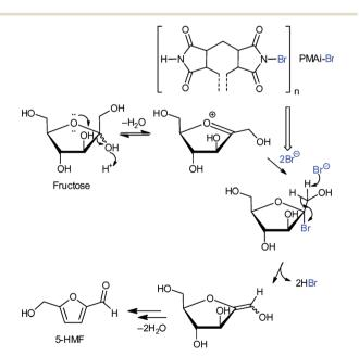
Fig. 16 Coordination of the N(-Br) atom of PMAi-Br as a polymer ligand to the Cr OMS in MIL-101Cr releases a bromide anion for a nucleophilic attack on the fructofuranosyl oxocarbenium ion according to the suggested mechanism for the fructose to 5-HMF dehydration. 122 Redrawn with permission from ref. 122.
