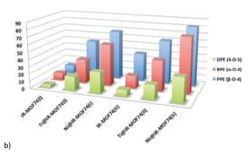
Fig. 33 (a) Pore diameters of IRMOF-74(I) and IRMOF-74(II) and largest intramolecular distances in the aromatic ether compounds, corresponding to a straight line between the blue-highlighted atoms in the optimized geometries. (b) Conversion efficiencies of the substrates into the corresponding hydrocarbon and phenol at 120 °C under 10 bar hydrogen. Reprinted with permission from ref. 166. Copyright 2016, American Chemical Society.
