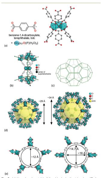
Fig. 8 (a) Ligand and metal building blocks in the trinuclear  $\{Cr_3(\mu_3-\mu_3)\}$  $O(O_2C-)_6(F/OH)(H_2O)_2$  building unit; (b) supertetrahedra; (c) mesoporous zeotypic network; (d) small cage with pentagonal windows and large cage with pentagonal and hexagonal windows; (e) dimensions of pentagonal and hexagonal cage window apertures. Objects in (a) to (e) are not drawn to scale. Graphics have been created from the deposited cif-file for MIL-101Cr (CSD-Refcode OCUNAK).51
