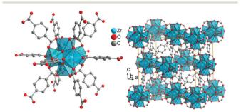
Fig. 9 Structure of zirconium terephthalate UiO-66Zr. The SBU is a hexanuclear and octahedral cluster of six edge-sharing ZrO<sub>8</sub> square antiprisms, which is connected to 12 neighboring SBUs in a face-centered cubic (fcc) packing arrangement. The structure was drawn from deposited cif-files under CCDC 837796 (UiO-66).<sup>81</sup>
