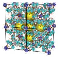
Fig. 19  $1 \times 2 \times 2$  super unit cell of NUS-6(Hf) with mesopores indicated by yellow spheres. Reprinted with permission from ref. 124. Copyright 2016, American Chemical Society.
