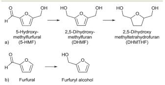
6 (a) Conversion of 5-HMF to 2.5-dihydroxymethyl-Scheme tetrahydrofuran (DHMTHF) and (b) conversion of furfural to furfuryl alcohol
