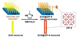
Fig. 7 Schematic illustration of ZnO@ZIF-8 patterns fabricated from the solid to MOF transformation. Reprinted from ref. 27 with permission from the American Chemical Society.
