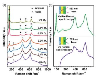
Fig. 2 (a) Visible Raman spectra of the  $TiO_2$  films fabricated at different  $O_2$  partial pressures. (b) Visible and UV Raman spectra of the  $TiO_2$ -AR electrode, which consists of an internal anatase phase  $TiO_2$  layer and external rutile phase  $TiO_2$  layer.
