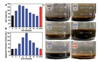
Fig. 6 (a) Yields of GO-n and GO-0-95, and (b) the apparent volumes of their GO precursors, (c) photographs of GO-n and GO-0-95 pastes; the values of n are depicted in the axis of (a) or (b), and in panel (c)
