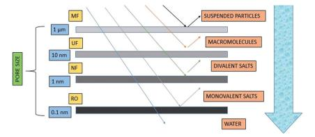
Fig. 4 Size of different particulates rejected by various membrane processes.<sup>32</sup>
