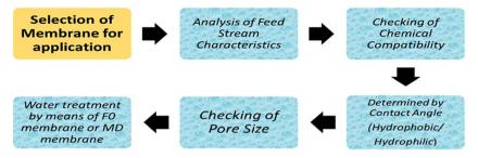
Fig. 11 Primary criteria for selecting the membrane for a water treatment process.
