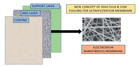
Fig. 12 Three-tier concept to fabricate high flux and low-fouling ultrafiltration membrane. [Note: plotted and modified by taking the figure from ref. 118.]
