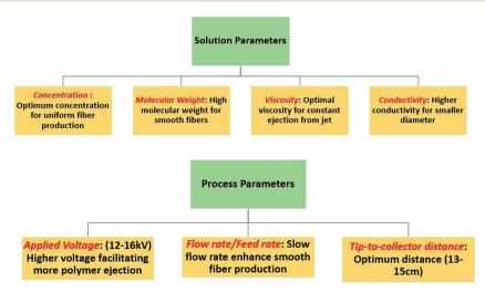
Fig. 7 Parameters affecting the electrospun nanofibrous membrane.
