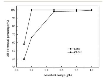
Fig. 5 Effect of adsorbent dosages on the removal of AB 14 by Mg–Al LDH and calcined Mg–Al LDH (adapted from ref. 33 with Copyright from 2013 Elsevier).
