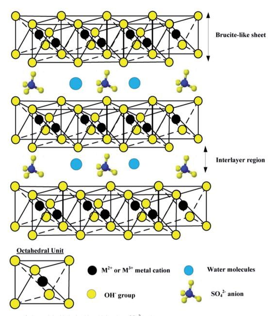
Fig. 1 The structure of a layered double hydroxide, with interlayer  $SO_4^{2-}$  anions.
