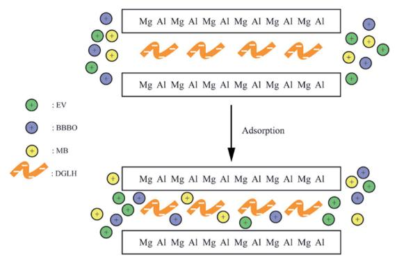
Fig. 11 The proposed adsorption mechanism for cationic dyes with DGLH-LDH.
