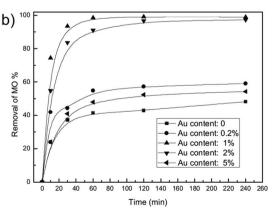
Fig. 7 Effect of material component on MO removal of Au/ZnAl LDO nanocomposites. (a) Different Zn content with constant Au content of 1% and (b) different Au content with constant Zn content of 87% (adapted from ref. 90 with Copyright from 2013 Elsevier).
