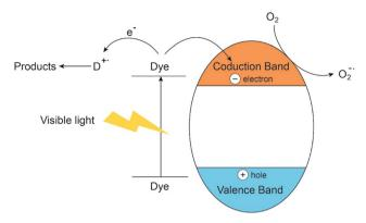
Fig. 13 Electron transfer process from the excitation of dye in the visible region.
