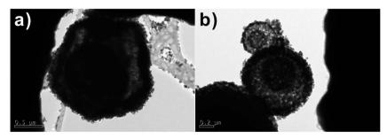
Fig. 7 TEM images of  $SnO_2$  samples after calcination at (a) 700 and (b) 500 °C with 1:1 molar ratio of sucrose and  $SnCl_4 \cdot 5H_2O$ .
