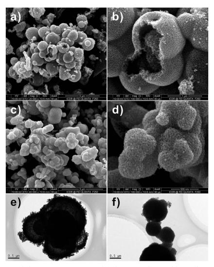
Fig. 6 FESEM and TEM images of  $SnO_2$  samples after calcination at 600 °C for 3 h with (a and b, e) 2:1 and (c and d, f) 1:2 molar ratio of polycose and  $SnCl_4 \cdot Sh_2O$ .
