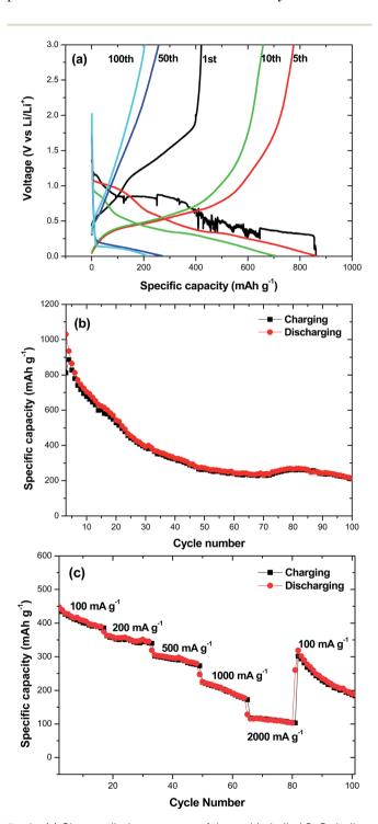
Fig. 8 (a) Charge–discharge curves of the multi-shelled  $SnO_2$  hollow sphere electrode for the  $1^{st}$ ,  $5^{th}$ ,  $10^{th}$ ,  $50^{th}$ , and  $100^{th}$  cycle at current density of 100 mA  $g^{-1}$ ; (b) the cycling performance of the multi-shelled  $SnO_2$  hollow spheres; (c) charge–discharge curves of the multi-shelled  $SnO_2$  hollow spheres at different current densities.
