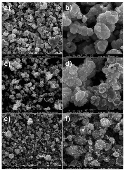
Fig. 1 FESEM images of SnO<sub>2</sub> samples after hydrothermal reaction at 180 °C with 1:2 molar ratio of p-glucose and metal salt. (a and b)  $Na_2SnO_3 \cdot 3H_2O$ , (c and d)  $SnCl_2 \cdot 2H_2O$  and (e and f)  $SnCl_4 \cdot 5H_2O$ .
