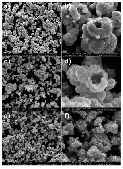
Fig. 2 FESEM images of SnO<sub>2</sub> samples after calcination at 550 °C for 3 h with 1:2 molar ratio of p-glucose and metal salt. (a and b) Na<sub>2</sub>-SnO<sub>3</sub>·3H<sub>2</sub>O, (c and d) SnCl<sub>2</sub>·2H<sub>2</sub>O and (e and f) SnCl<sub>4</sub>·5H<sub>2</sub>O.
