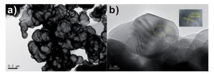
Fig. 4 (a) TEM (b) HRTEM images of  $SnO_2$  samples after calcination at 550 °C for 3 h with 1 : 2 molar ratio of p-glucose and  $SnCl_2 \cdot 2H_2O$ .
