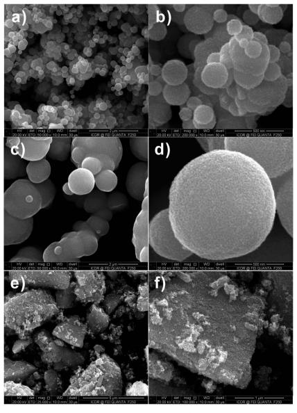
Fig. 3 FESEM images of SnO<sub>2</sub> samples after calcination at 550 °C for 3 h with 1:0.4 molar ratio of p-glucose and metal salt. (a and b) Na<sub>2</sub>- $SnO_3 \cdot 3H_2O$ , (c and d)  $SnCl_2 \cdot 2H_2O$  and (e and f)  $SnCl_4 \cdot 5H_2O$ .
