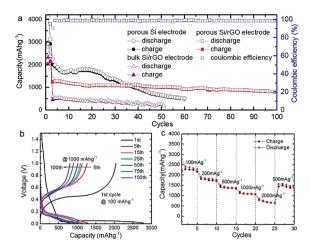
Fig. 15 (a) Cycle performance at a constant current rate of 1000 mA  $\rm g^{-1}$  after initial activation processes at 100 mA  $\rm g^{-1}$  for two cycles; (b) galvanostatic discharge–charge profiles; and (c) rate performance of Si/graphene composite electrode.<sup>171</sup> Reprinted (adapted) with permission from ref. 171. Copyright (2015) American Chemical Society.
