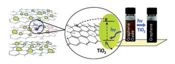
Fig. 13 Photo catalyst electron acceptance by GO and change in color from brown to black after GO reduction.<sup>137</sup> Reprinted (adapted) with permission from ref. 137. Copyright (2008) American Chemical Society.
