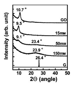
Fig. 8 XRD patterns of GO, graphite (G), and rGO obtained using various molar concentrations of NaBH<sub>4</sub>.  $^{97}$  Reprinted (adapted) with permission from ref. 97. Copyright © 2009 WILEY-VCH Verlag GmbH & Co. KGaA, Weinheim.
