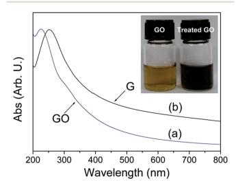
Fig. 14 UV visible absorption spectra of the GO (a) before and (b) after hydrothermal treatment at 180  $^{\circ}$ C for 6 h. Inset shows the color change of 0.5 mg mL $^{-1}$  GO solution before and after hydrothermal treatment. Reprinted (adapted) with permission from ref. 147. Copyright (2009) American Chemical Society.
