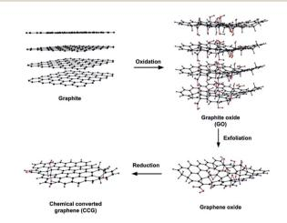
Fig. 7 Preparation of chemically converted graphene (CCG) by reduction of GO.<sup>96</sup> Reprinted (adapted) with permission from ref. 96. Copyright © 2011 WILEY-VCH Verlag GmbH & Co. KGaA, Weinheim.
