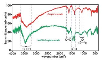
**Fig. 6** FTIR spectra of graphite oxide and NaOH-graphite oxide.<sup>78</sup> Reprinted (adapted) with permission from ref. 78. Copyright (2010) American Chemical Society.
