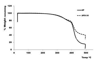
Fig. 4 Thermogravimetric analysis curves for the AP and APD-30 composite
