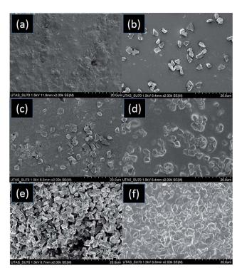
Fig. 2 SEM images taken from a cross-section of (a) AP (b) APD-10 (c) APD-20 (d) APD-25, and (e)-(f) APD-30 composite materials.
