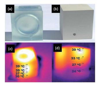
Fig. 8 (a) 3D printed heating coil using commercial resin, (b) 30% (w/v) composite material, (c) IR images of polymer heating coil containing hot water introduced at 40  $^{\circ}$ C (d) IR image of composite heating coil containing hot water introduced at 40  $^{\circ}$ C.
