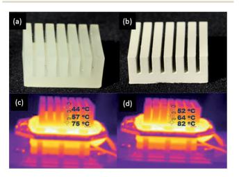
Fig. 7 (a) 3D printed heat sink using commercial acrylate resin, (b) 3D printed heat sink using 30% (w/v) composite material, (c) IR images of polymer heat sink heated for 10 min at 100  $^{\circ}$ C, (d) IR image of composite heat sink heated for 10 min at 100  $^{\circ}$ C.
