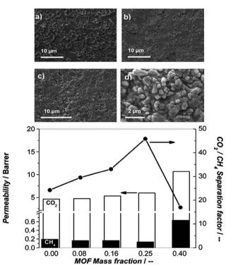
Fig. 13 SEM micrographs of the cross section of mixed matrix membrane containing 8 (a), 16 (b), 25 (c) and 40 (d) wt% NH $_2$ -MIL-53(Al) crystals. Reprinted from ref. 92 with permission from Royal Society of Chemistry.
