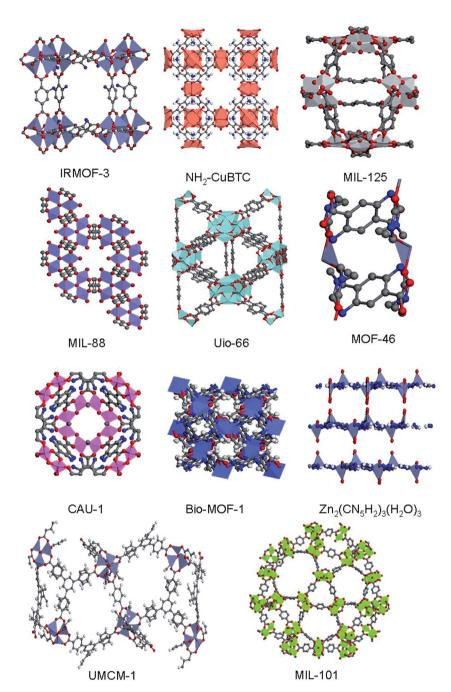
Fig. 1 Structures/cages of amine-functionalized MOFs or their parents.
