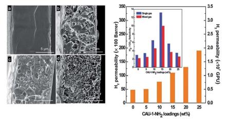
Fig. 14 Left: SEM images of the cross section of pure poly(methyl methacrylate) membrane (a) and MMMs with 5 wt% (b), 15 wt% (c) and 25 wt% (d) CAU-1 loading. Right:  $H_2$  permeability of the MMMs with different CAU-1 loadings and the corresponding  $H_2/CO_2$  selectivities (inset). Reprinted from ref. 95 with permission from Royal Society of Chemistry.
