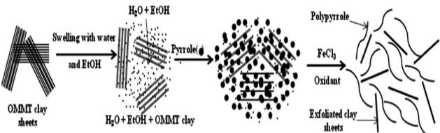
Fig. 7 The formation of exfoliated PPy-OMMTC nanocomposites. 123
