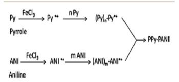
Scheme 4 The polymerization of pyrrole and aniline monomers, and the formation of PPy-PANI nanofibers.<sup>33</sup>
