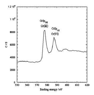
Fig. 4 The XPS spectra of the PPy/Fe<sub>3</sub>O<sub>4</sub> nanocomposites after Cr(v<sub>1</sub>) adsorption.113
