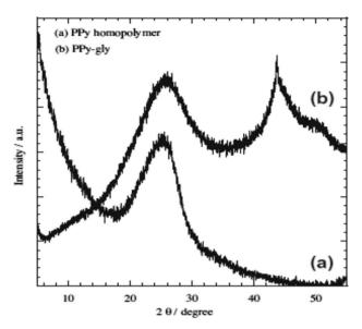
Fig. 3 XRD curves of (a) PPy homopolymer and (b) PPy-gly.<sup>38</sup>
