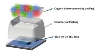
Fig. 1 Sketch of WHLEDs based on a blue- or UV-LED with organic down-converting packings.
