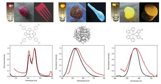
Fig. 3 Upper part – pictures of an exemplary of the gels (room light, with a magnetic stirrer) and rubber materials with compounds 3, 4, and 7 prepared in a ball-like shape (room light) and onto irregular 3D surfaces ( $\lambda_{exc}$  = 310 nm), such as kitchen forks, glass pipette, and plastic vial cap. Central part – chemical structures of compounds 3, 4, and 7. Bottom part - emission spectra of the luminescent compounds in solution (black) and rubbers (red).
