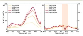
Fig. 3 Change in the absorption spectra of SNO thin crystals measured 28 ms after excitation for different number of 266 nm laser shots (1.4 mJ cm<sup>-2</sup>) a) without using the NOPA photoreversion pulse and b) with the photoreversion pulse (2.8 mJ cm<sup>-2</sup>). The spectral region covered by the NOPA is shaded. In this region, the scattered light coming from the NOPA beam reaching the detector produced fluctuations increasing the noise significantly.
