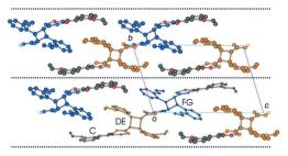
Fig. 11 Crystal packing of the structure determined after 60 h of UV exposure (67% conversion) at 343 K as viewed down the a axis.
