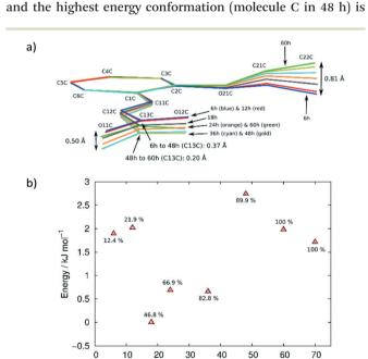
Fig. 7 (a) Superimposition of C molecules from the 6, 12, 18, 24, 36, 48 and 60 h structures by least squares fit of corresponding phenyl (C1C-C6C) atoms. (b) Relative energies of the C molecules at different reaction times. Indicated next to each point is the degree of conversion in the AB site.
