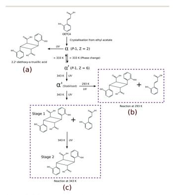
Scheme 1 Different reaction pathways which can be explored starting from the  $\alpha$  polymorph of OETCA; a) reaction product from the  $\alpha$  polymorph; b) 293 K reaction product of the  $\alpha'$  polymorph (obtained by phase transition of the  $\alpha$  polymorph at 333 K); 15,29 c) reaction of the  $\alpha'$  polymorph at 343 K (this work).
