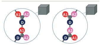
Fig. 2 Competition of two different H-bond acceptors (A1 and A2) for one H-bond donor (D) in the solid state. The difference in the stabilities of the two different H-bonds determines the probability of formation
