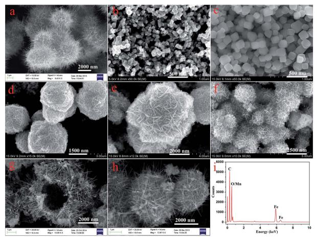
Fig. 1 SEM images of as-prepared nanostructures. (a) MnO<sub>2</sub>; (b) Fe<sub>3</sub>O<sub>4</sub>; (c) Fe<sub>2</sub>O<sub>3</sub>; (d)-(g) Fe<sub>3</sub>O<sub>4</sub>@MnO<sub>2</sub> prepared at times of 3 h, 6 h, 9 h, and 15 h, respectively; (h) Fe<sub>2</sub>O<sub>3</sub>@MnO<sub>2</sub> prepared at time of 6 h; (i) typical EDXS of Fe<sub>3</sub>O<sub>4</sub>@MnO<sub>2</sub> nanocomposites prepared at 6 h.
