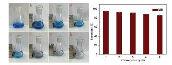
Fig. 7 Regeneration studies of as-prepared  $Fe_3O_4@MnO_2$  nanocomposites in the removal of MB. The photographs showed the MB solution (a) and adsorption process under magnetic separation at different time intervals ((b)–(h) 0, 10, 20, 30, 40, 50, and 60 min).
