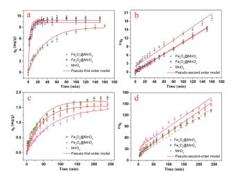
Fig. 6 Adsorption kinetics curves of as-prepared  $Fe_3O_4@MnO_2$  and  $Fe_2O_3@MnO_2$  nanocomposites onto MB (a and b) and RhB (c and d) at 298 K.
