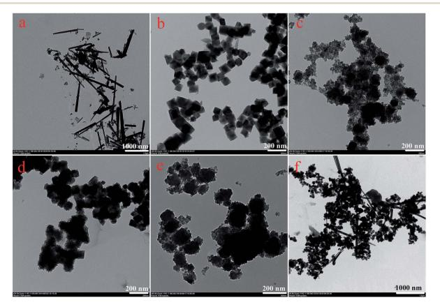
Fig. 2 TEM images of as-prepared nanostructures. (a),  $MnO_2$ ; (b),  $Fe_3O_4$ ; (c)–(f),  $Fe_3O_4$ @ $MnO_2$  nanocomposites prepared at times of 3 h, 6 h, 9 h, and 15 h, respectively.
