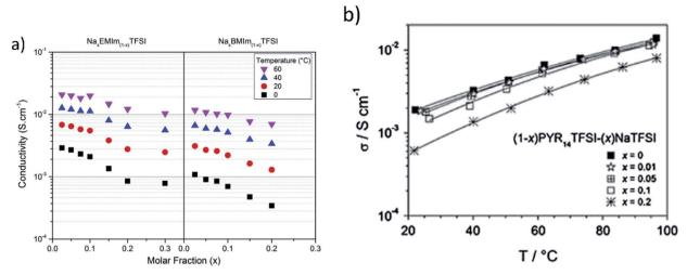
Fig. 18 (a) Isotherms of the conductivity as a function of the molar fraction of  $Na_x$ -EMIm $_{(1-x)}$ TFSI and  $Na_x$ BMIm $_{(1-x)}$ TFSI (reproduced with permission<sup>153</sup> © 2014, Elsevier) and (b) ionic conductivity vs. temperature for the (1-x)PYR $_{14}$ TFSI-(x)NaTFSI electrolyte. Reproduced with permission<sup>154</sup> © 2014, Elsevier.
