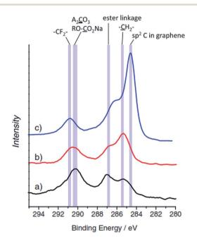
Fig. 20 XPS carbon 1s spectra for the hard-carbon electrodes tested in (a) sodium and (b) lithium cells after the first cycle, and (c) pristine electrode. Reproduced with permission  $^{128}$  © 2011, WILEY-VCH Verlag GmbH & Co.
