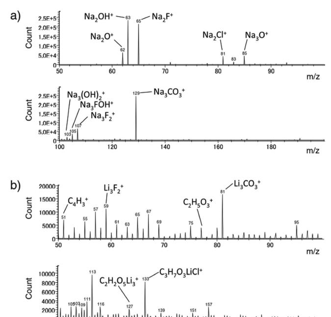
Fig. 21 TOF-SIMS positive ion spectra for the hard-carbon electrodes after the first galvanostatic cycle in (a) sodium and (b) lithium cells. Reproduced with permission<sup>128</sup> © 2011, WILEY-VCH Verlag GmbH & Co
