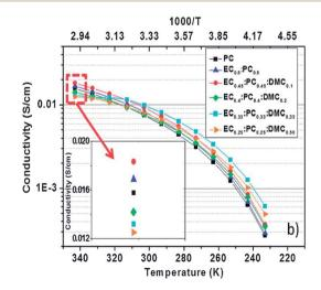
Fig. 16 Arrhenius plots of the conductivity of the electrolyte based on 1 M NaTFSI salt dissolved in various solvent mixtures. Reproduced with permission<sup>152</sup> © 2013, RSC Publishing
