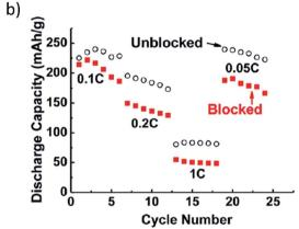
Fig. 13 (a) Na ions transport along and diffuse through the mesoporous wood fiber structure. Internal transport pathways are blocked by the conformal  $Al_2O_3$  coating, and (b) the rate performance of the Sn anode deposited on the carbon-coated mesoporous wood fibers. Reproduced with permission<sup>137</sup> © 2013, ACS Publications.
