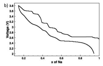
Fig. 4 Voltage profiles: (a) Na<sub>x</sub>MnO<sub>2</sub> cycled at C/10 with the cycle numbers indicated, and (b) Na<sub>x</sub>MnO<sub>2</sub> de/sodiation as measured by potentiostatic intermittent titration. Reproduced with permission<sup>36</sup> © 2012, The Electrochemical Society.
