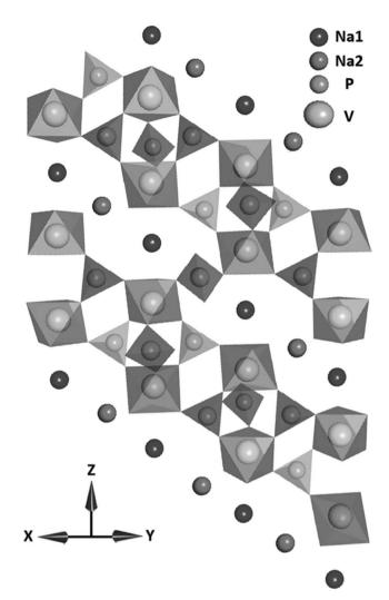
Fig. 9 The crystal structure of  $Na_3V_2(PO_4)_3$  in the a and b plane. Reproduced with permission<sup>81</sup> © 2013, WILEY-VCH Verlag GmbH & Co.
