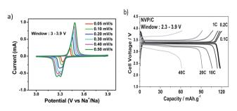
Fig. 10 (a) Cyclic voltammogram of  $Na_3V_2(PO_4)_3$ , and (b) galvanostatic charge and discharge profiles for several C rates. Reproduced with permission<sup>81</sup> © 2013, WILEY-VCH Verlag GmbH & Co.
