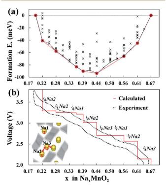
Fig. 6 (a) Formation energies of seven stable intermediate phases during  $Na_xMnO_2$  cycling calculated from 156 different sodium configurations, and (b) experimental and calculated voltage profiles for  $Na_xMnO_2$  with respect to the minimum energy path of formation energies. Reproduced with permission<sup>35</sup> © 2012, ACS Publications.
