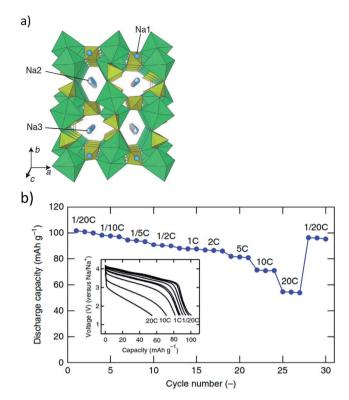
Fig. 8 (a)  $Na_2Fe_2(SO_4)_3$  structure projected along the c axis, and (b) capacity retention upon cycling up to 30 cycles under various rate of C/20 (2 Na in 20 h) to 20 C. Reproduced with permission<sup>80</sup> © 2014, Nature Publishing Group.
