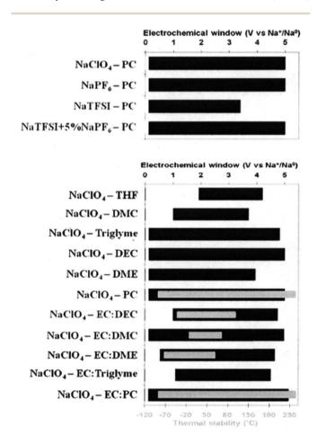
Fig. 15 Electrochemical potential window stability of various salts with PC and NaClO<sub>4</sub> in various solvents. Reproduced with permission<sup>150</sup> © 2012, RSC Publishing
