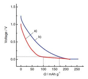
Fig. 19 Chronopotentiograms of the second reduction for hard-carbon electrodes in (a) 1 mol dm $^{-3}$  NaClO $_4$  and (b) 1 mol dm $^{-3}$  LiClO $_4$  PC solution in Na and Li cells, respectively, at a rate of 25 mA g $^{-1}$ . Reproduced with permission  $^{128}$  © 2011, WILEY-VCH Verlag GmbH & Co.
