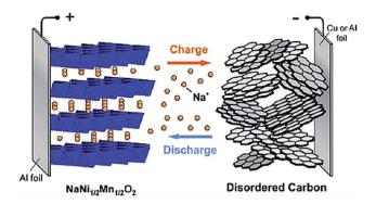
Fig. 2 Schematic of sodium ion batteries with a layered transition metal oxide cathode and carbonaceous anode. Reproduced with permission<sup>23</sup> © 2011, ACS Publications.
