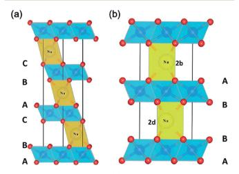
Fig. 3 The crystal structure of (a) O3 and (b) P2 phases in  $A_xMO_2$  Reproduced with permission<sup>4</sup> © 2013, RSC Publishing.
