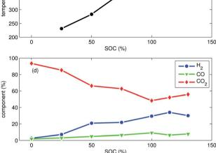
Fig. 5 Summary of all experiments with LFP cells at different SOC: (a) onset cell temperature  $\theta_{o}$ . (b) Maximum cell temperature  $\theta_{m}$ . (c) Amount of produced gas  $n_{\text{sum}}^{\text{ideal}}$ . (d) Main detected gas components  $r_i^{\text{GC}}$ .
