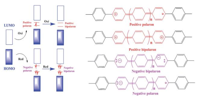
Fig. 4 Design of polyphenylene electronic and chemical structural changes during (a) oxidation (p-doping) and (b) reduction (n-doping). A radical cation (positive polaron) is formed *via* oxidation, while a radical anion (negative polaron) is formed during reduction. High states of charge can lead to the formation of positive and negative bipolarons. Cations and anions counterbalance charges in the polymer chain.
