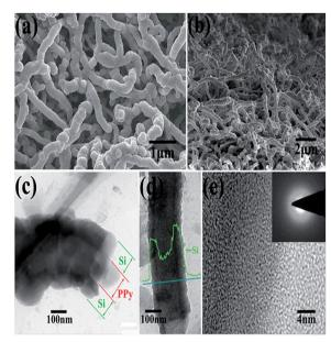
Fig. 8 (a) and (b) top and cross-sectional SEM images of PPy–Si coreshell nanofiber network after Si deposition. (c) and (d) TEM images of the core–shell structure of Si@PPy nanocables. (e) High-resolution TEM image of Si coatings. Inset of (e) SAED image of Si coatings (reprinted with permission from ref. 186, copyright 2012, Royal Society and Chemical Journal).
