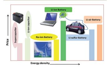
Fig. 1 Plot of price vs. energy density for different energy storage systems.
