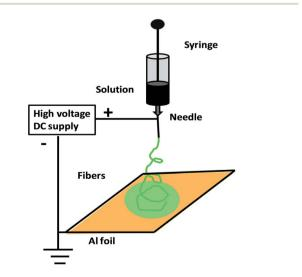
Fig. 3 Schematic of electrospinning method for the synthesis of conductive polymer nanofibers.
