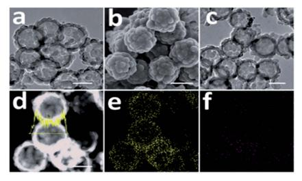
Fig. 10 (a) TEM image of T-HSSP, (b) SEM image of T-HSSP, (c) TEM image of S@PPy-300 composite, (d) STEM image and line scan analysis (sulfur) of S@PPy-300 composite, (e) elemental mapping of sulfur in (d) and (f) elemental mapping of carbon in (d). All scale bars: 200 nm (reprinted with permission from ref. 244, copyright 2014, Royal Society and Chemical Journal).
