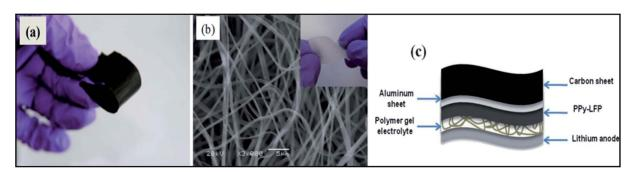
Fig. 7 Photograph (a) of a flexible PPy–LFP electrode, (b) SEM of electrospun P(VdF-HFP) matrix and (c) scheme of the flexible battery. Inset of (b) Photograph of electrospun P(VDF-HFP). (Reprinted with permission from ref. 161, copyright 2012, Royal Society and Chemical Journal).
