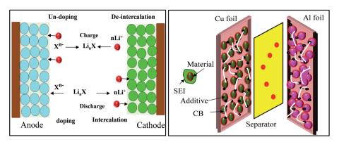
Fig. 2 Principle of LIBs based on doping/dedoping (negative) and deintercalation/intercalation (positive) electrodes and a model of the electrodes with their SEI system.
