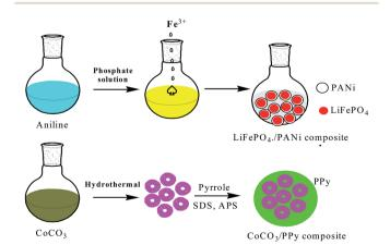
Fig. 5 Design of LiFePO $_4$ /carbon and CoCO $_3$ /PPy composites including an *in situ* polymerization reaction and two typical restriction processes.
