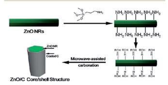
Fig. 21 Mechanism of formation of a carbon-coated ZnO core-shell structure (reprinted with permission from ref. 280; Copyright 2009 @ American Chemical Society).
