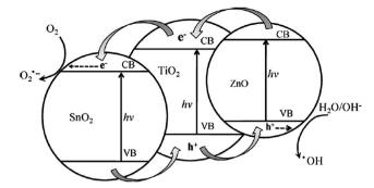
Fig. 14 Energy band structure and electron-hole separation process of a tri-component  $SnO_2$ - $TiO_2$ -ZnO system (reprinted with permission from ref. 227; Copyright 2012 @ Elsevier).
