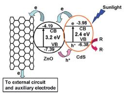
Fig. 25 Charge carrier separation and transportation in a CdS–ZNWs–MWCNTs heterojunction (reprinted with permission from ref. 311; Copyright 2011 @ Elsevier).
