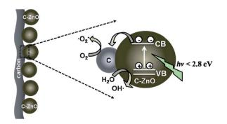
Fig. 19 Schematic presentation of doped and surface carbon in C-ZnO. The grey colour part indicates that the polymer nanowires are turned into carbon and olive colour spheres, representing C-ZnO (reprinted with permission from ref. 274; Copyright 2013 @ Royal Society of Chemistry).
