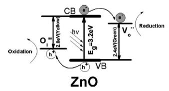
Fig. 3 Band structure and charge transfer pathways of ZnO nanocrystal with oxygen defects (reprinted with permission from ref. 81; Copyright 2009 @ American Chemical Society).
