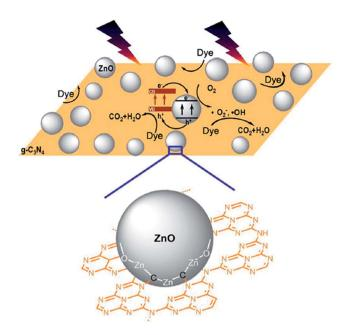
Fig. 24 Illustration of the electron–hole separation, transport, and photocatalytic progress of C–ZnO:g– $C_3N_4$  under visible light (reprinted with permission from ref. 310; Copyright 2014 @ American Chemical Society).
