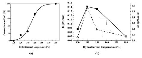
Fig. 15 (a) Phase transformation from  $ZnO_2$  to  $ZnO_3$  (b) rate constant (k) and normalized rate constant (k/x) vs. hydrothermal temperature (x is the  $ZnO_2$ -to-ZnO conversion) for the degradation of MO (reprinted with permission from ref. 242; Copyright 2005 @ Elsevier).
