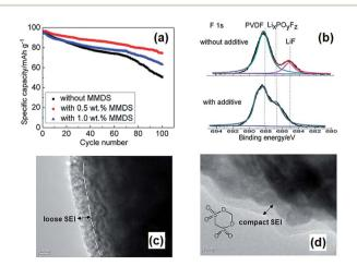
Fig. 5 (a) Discharge capacity retention of LMO/graphite full cell at 60 °C. (b) F 1s XPS spectra of LMO cathoes after 100 cycles at 60 °C. TEM images of LMO cathode surface cycled in (c) the additive-free electrolyte, (d) the MMDS-added electrolyte. Reproduced with permission.  $^{56}$
