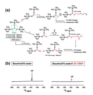
Fig. 19 (a) Proposed mechanisms for electrochemical oxidative decomposition of TMSP and for the unique function of TMSP scavenging HF from the electrolyte. (b) <sup>19</sup>F NMR spectra of the electrolyte with and without TMSP. Reproduced with permission.<sup>92</sup>
