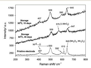
Fig. 10 Ex situ Raman spectra obtained from the pristine  $LiNi_{0.5}Mn_{1.5}O_4$ , the electrode stored at 30 °C for 15 days, and the electrode stored at 60 °C for 45 days in EC/DMC (1/2)/1.5 M LiPF<sub>6</sub>. Reproduced with permission.<sup>69</sup>
