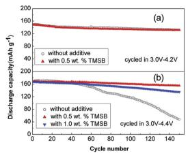
Fig. 8 Cycling performance of LiNi $_{0.5}$ Co $_{0.2}$ Mn $_{0.3}$ O $_2$ /graphite cells cycled at a rate of 1 C in the voltage ranges of (a) 3.0-4.2 V and (b) 3.0-4.4 V. Reproduced with permission. $^{57}$
