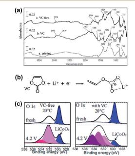
Fig. 4 (a) FTIR spectra obtained from the LMO cathodes before and after being cycled in the VC-free and VC-added electrolytes. (b) Possible mechanism of the VC decomposition. The polymerization of VC may occur by the radical species. (c) O 1s XPS spectra of the LCO cathodes before and after being cycled in the VC-free and VC-added electrolytes. Reproduced with permission.<sup>4,53</sup>
