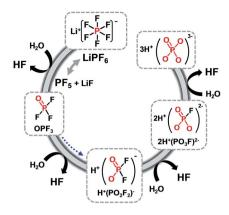
Fig. 18 Hydrolysis reactions of LiPF $_6$  salt in the presence of trace water in the cell.
