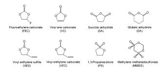
Fig. 1 Chemical structures of various organic-based additives
