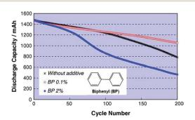
Fig. 6 Cycle life of  $LiCoO_2$ /graphite cylindrical cells with and without BP additive cycled between 2.7 V and 4.3 V at 45 °C. Reproduced with permission.<sup>26</sup>
