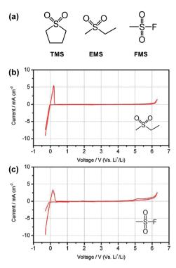
Fig. 14 (a) Structures of typical sulfone solvents. Cyclic voltammograms of 1 M LiPF<sub>6</sub> in (b) EMS/DMC (1:1 by wt) and (c) EMS/FMS (1:1 by wt). Scan rate: 5 mV s<sup>-1</sup>. Pt as the working and counter electrodes and Li as the reference electrode. Reproduced with permission.<sup>78</sup>
