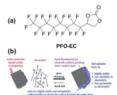
Fig. 25 (a) Chemical structure of PFO-EC. (b) Schematic for the formation of double-layer passivation films by decomposition of the head group on the cathode (or anode) surface forming an inner layer and self-assembly of tails on these inner layers forming a solvophobic outer layer. Reproduced with permission.<sup>117</sup>
