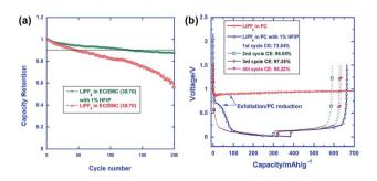
Fig. 20 (a) Cycling performance of LiNi $_{0.5}$ Mn $_{1.5}$ O $_4$  in the reference and HFiP-containing electrolytes. Percent capacity retention is shown for easy comparison. (b) Voltage profiles of the graphite anodes in the PC-based electrolyte with and without 1% HFiP additive. Reproduced with permission. <sup>96</sup>
