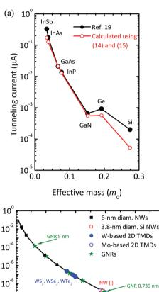
Transmission coefficient 10 10 10-10 MoS., MoSe., MoTe 0.2 0.4 0.6 0.8 1.0 Effective mass  $(m_0)$ Fig. 14 Tunneling behavior of 5 nm wide source-drain barriers. (a)
