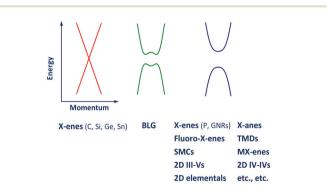
Fig. 7 Schematic band structure of 2D materials relevant for transistors. BLG: bilayer graphene; GNR: graphene nanoribbon; TMD: transition metal dichalcogenide; SMC: semimetal chalcogenide
